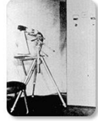
The first mammography system was essentially a tripod supporting a special X-ray camera
