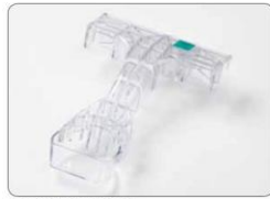
7.5 cm Spot Contact Paddle Diagnostic D-shaped spot compression paddle used for diagnostic views. This paddle shifts utilizing the right and left portions of the digital detector during oblique and lateral views. Part number: ASY-01986
