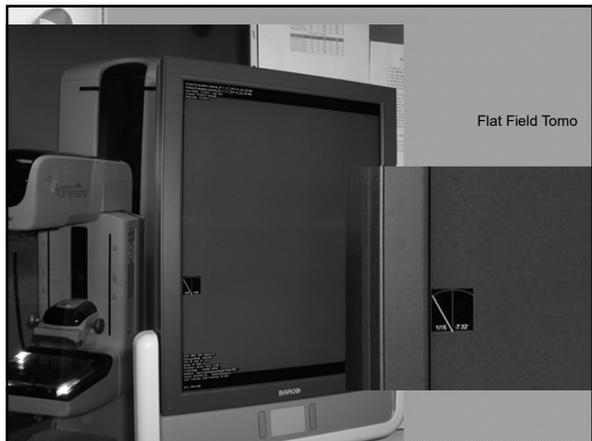
*Artifacts that appear on the Flat Field phantom provided by the manufacturer must not be overlooked. Such artifacts will have an impact on detector calibration since the same block is being used during detector calibration. Replacement of the Flat Field phantom must be considered.*
